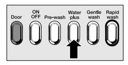
■ Press the "Water plus" button 4 times (i.e. press in and out twice)
